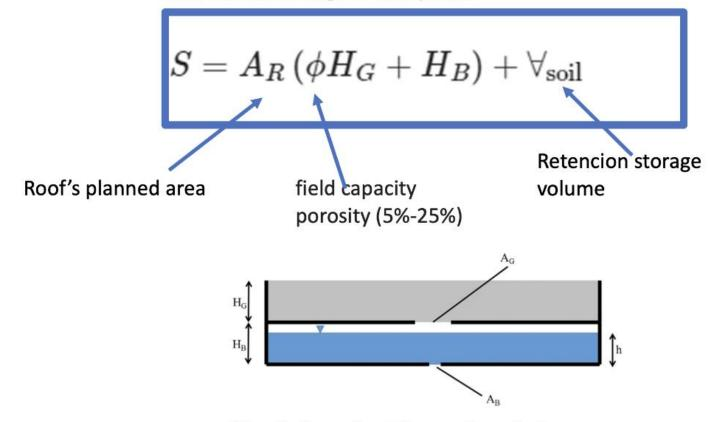
Schematic diagram of a modular green-blue roof system.  $A_G = \sum A_{Gi}$  and  $A_B = \sum A_{Bi}$  are the cumulative drain areas of the green roof and blue roof, respectively.  $H_G$  and  $H_B$  are the heights of the green roof and blue roof modules, and h is the height of water at time *t* in the blue roof module
