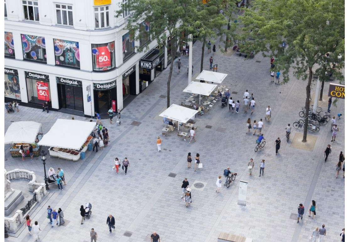
Change of materials, reduction of speed, narrowing the lane, addition of furniture
